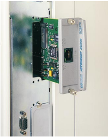
HP Color LaserJet 8500 DN model comes with two available EIO slots and parallel connector.
